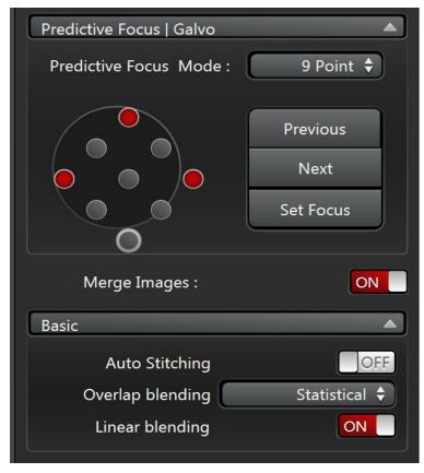
Images is ON, Auto Stitching is OFF, Overlap Blending is set to Statistical, and Linear Blending is ON. Then click on the START button at the bottom right of the software to begin capturing your tiled image.
