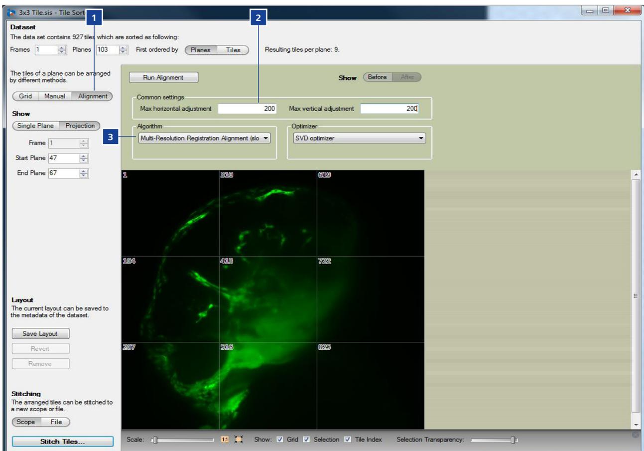
Figure 5 Steps for automatic alignment of tiled image stacks
